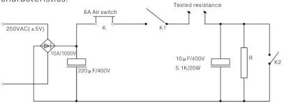
As shown in the figure: close the air switch K. Disconnect K2, will K1 repeated on and off 10000 times, the resistor does not open circuit.
